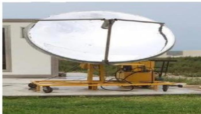
Figure 1: Installation of parabolic solar collector.
